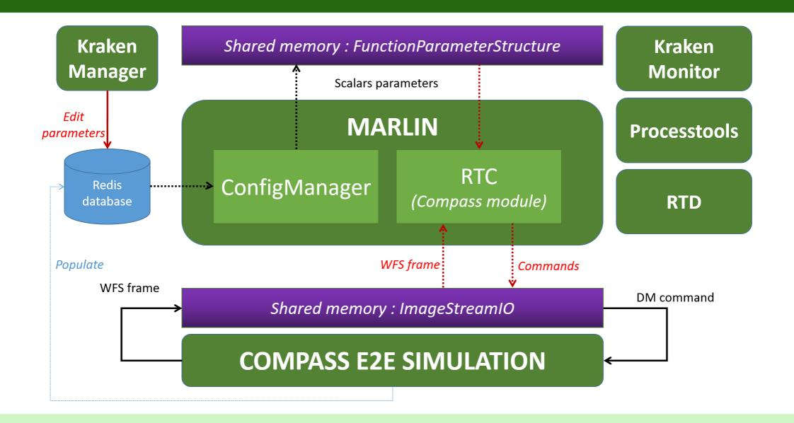
Validation made with E2E simulation tool COMPASS
